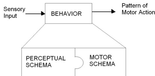
The motor schema can be described by the **potential fields methodology** where the robot feels the vector force by summing the magnitude and direction of the sensor data.
