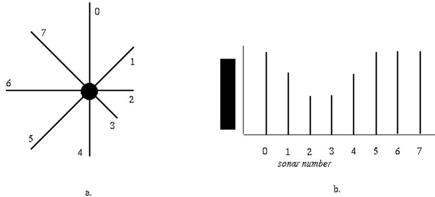
This sonar polar plot can be used to implement run away, wander, and follow corridor reactive rules. For level 0, if the polar plot indicates that the robot hit an object then it should stop moving. The polar plot is also used to determine the strength of the force from the object to generate a turn angle to move the robot away and then move forward.
